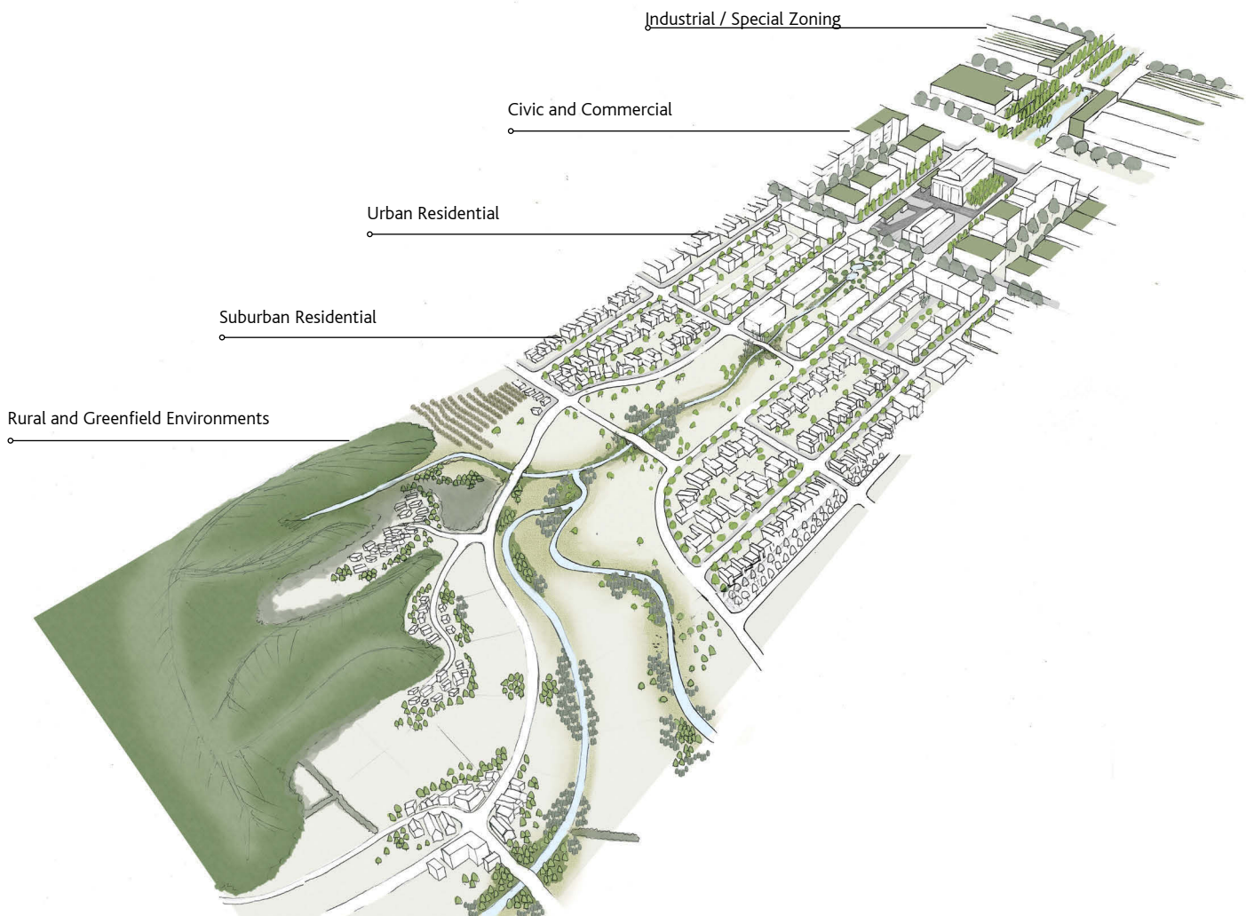
Figure 23: The 'urban transect' demonstrates an increase in urban activity and imperviousness, requiring a corresponding design approach for stormwater management and ecosystem services.
