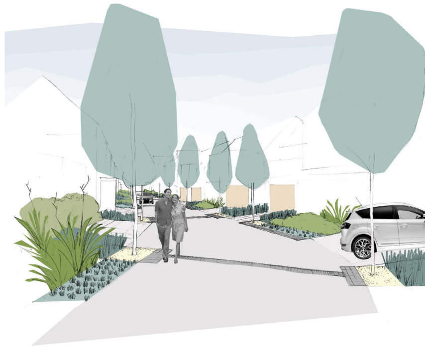
Figure 31: Laneways combine pedestrian and automobile surfaces, providing primary treatment of stormwater and operating as overland flow paths.
