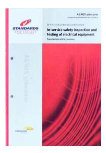
AS/NZS 3760 covers the in-service safety inspection and testing of low voltage (single phase and polyphase) portable electrical equipment.
