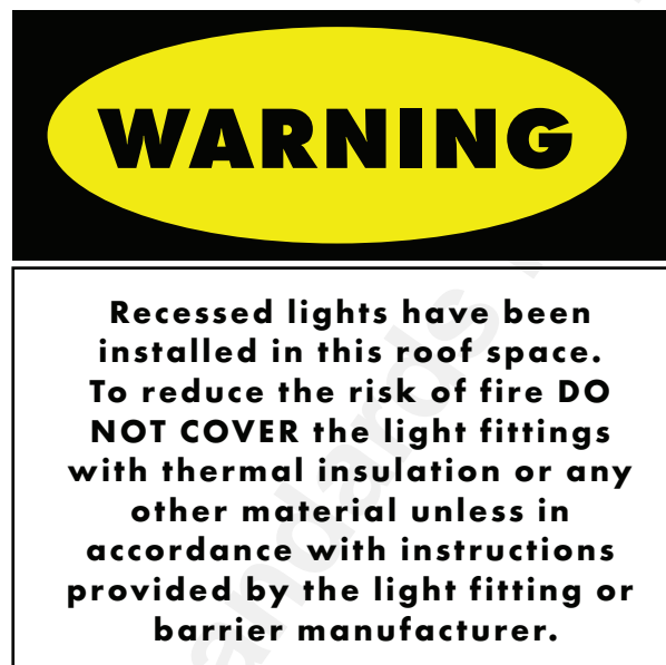
FIGURE 4.10 WORDING FOR WARNING SIGN TO BE INSTALLED IN ACCESSIBLE ROOF SPACES CONTAINING RECESSED LUMINAIRES
