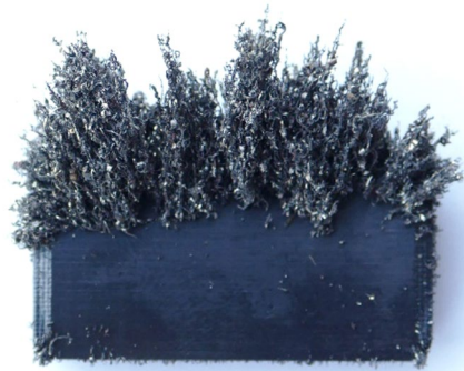
Iron swarf lining up with magnetic flux
