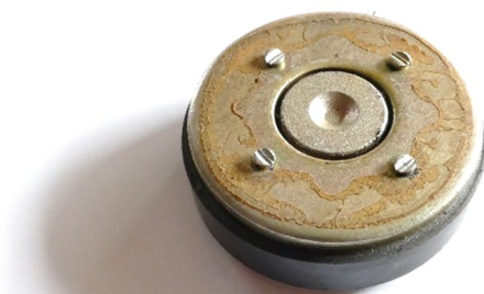
Magnet pulled off a speaker showing the circular slot in the magnet
