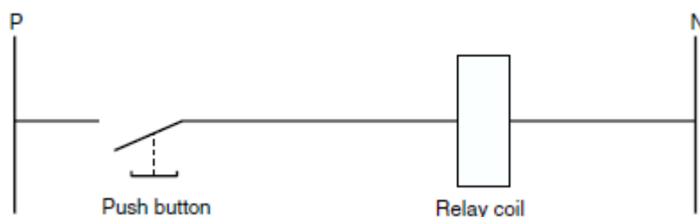
Figure 15: Push button control on/off
