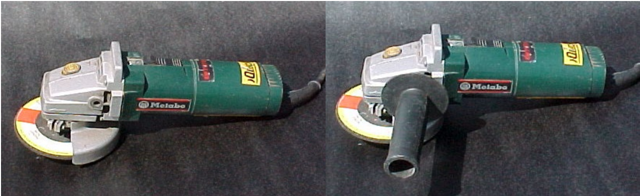
The handle, which can be fitted either side; is missing altogether
